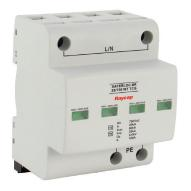
Location of Use: Main Distribution Boards Network Systems: TN-S, TN-C, TT (only L-N) Mode of Protection: L-PE, N-PE, L-PEN, L-N Surge Ratings:  $I_{imp} = 25 \text{ kA} (10/350 \,\mu\text{s})$  $I_{max} = 80 \text{ kA} (8/20 \,\mu\text{s})$
